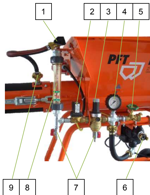
Fig. 3: Water Manifold with Water pressure booster pump
