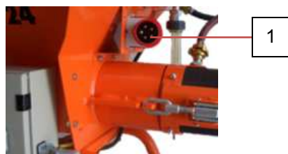
Fig. 7: Electrical connection
