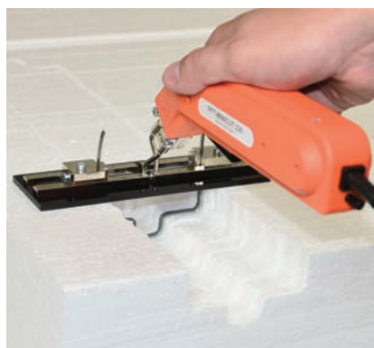
Free selectable forms, e. g. slot cuttings caused by simple bending of the cutting strap.
