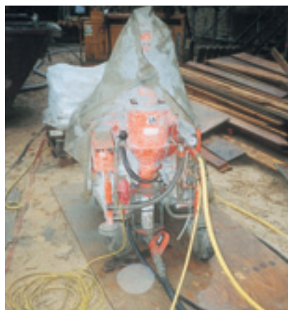
The PFT G 4 mixing pump proved its flexibility: During this restoration job, it was used to pressure-grout drill holes, fill cavities and apply a historical-style exterior plaster.
