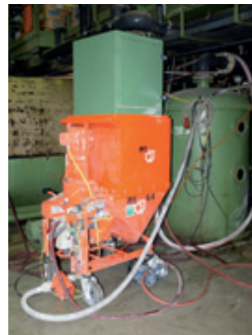
Semi-mobile operation of the modified PFT G 4 mixing pump in the initial testing phase.
