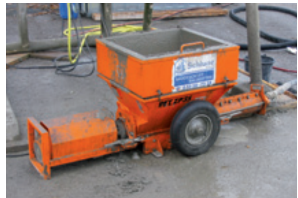
The PFT ZP 3 S pump conveyed the 8 mm shotcrete used.
