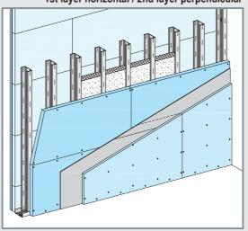
Cladding 3x 12.5 mm + sheet steel layer ≥ 0.5 mm
