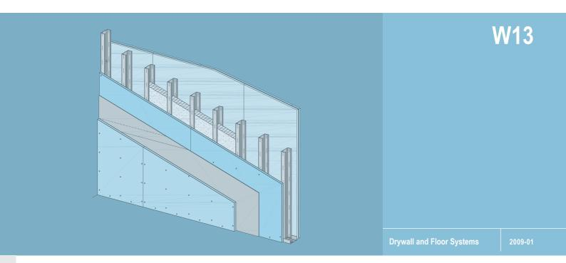
W131 – Knauf Fire Wall - Single metal stud frame double- or triple-layer cladding with sheet steel layer
