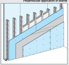
Cladding 20 + 12.5 mm + sheet steel layer ≥ 0.5 mm
