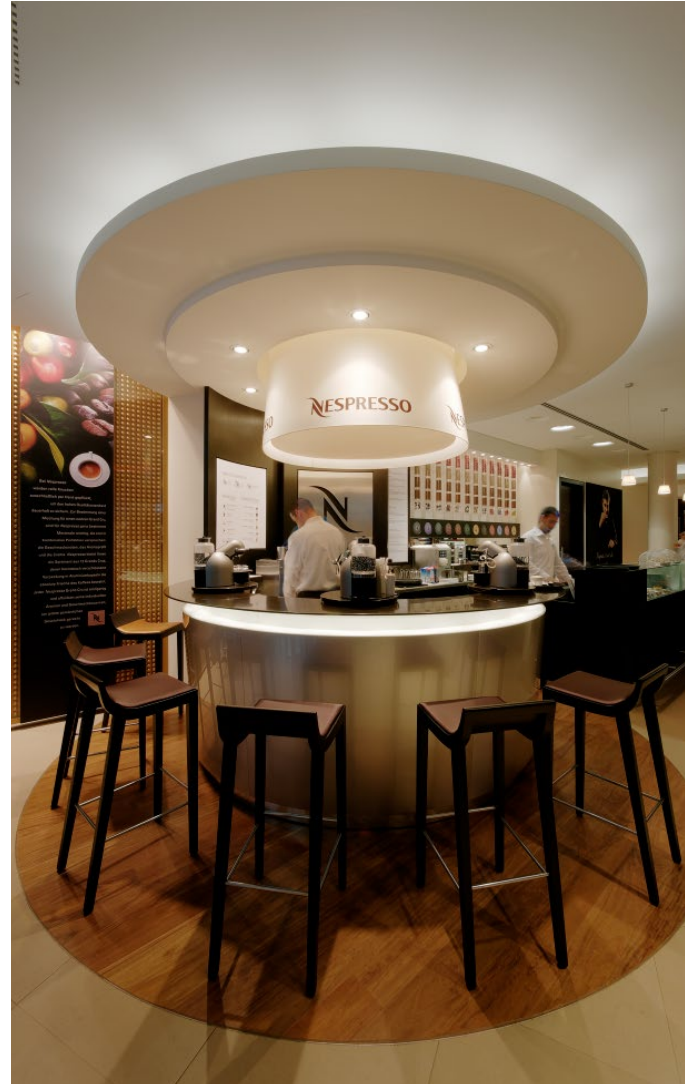
Ceiling construction of the shop - The ceiling is suspended via many layers, the lighting is integrated and plastered in.
