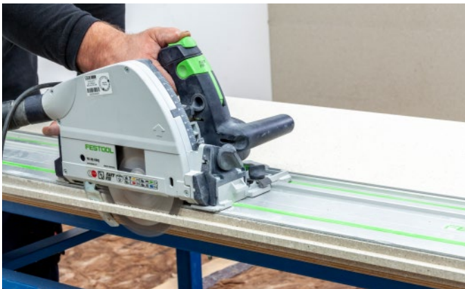
Bild 11: Cut wall connection element
