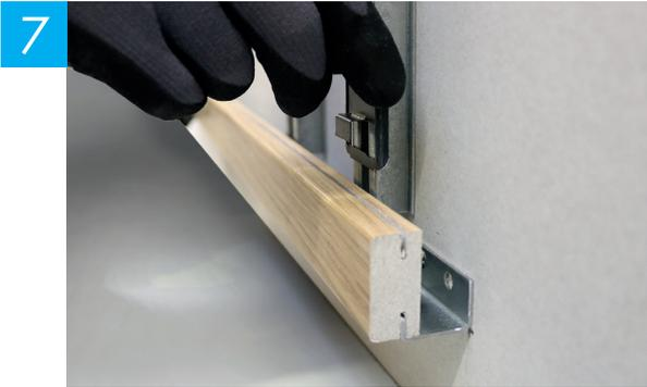
Force lock the DESIGNLINE using the KDLF twist clip pushed down into place.
