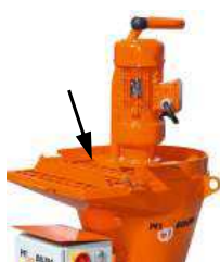
Fig. 27: Fill in water
