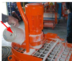
Fig. 34: Fill in water
