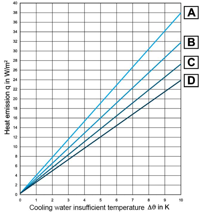
A:  $R_{\lambda,B} = 0,00$  (without floor finishing) B:  $R_{\lambda,B} = 0,05$  (with e.g. porcelain stoneware) C:  $R_{\lambda,B} = 0,10$  (with e.g. laminate flooring) D:  $R_{\lambda,B} = 0,15$  (with e.g. carpet)
