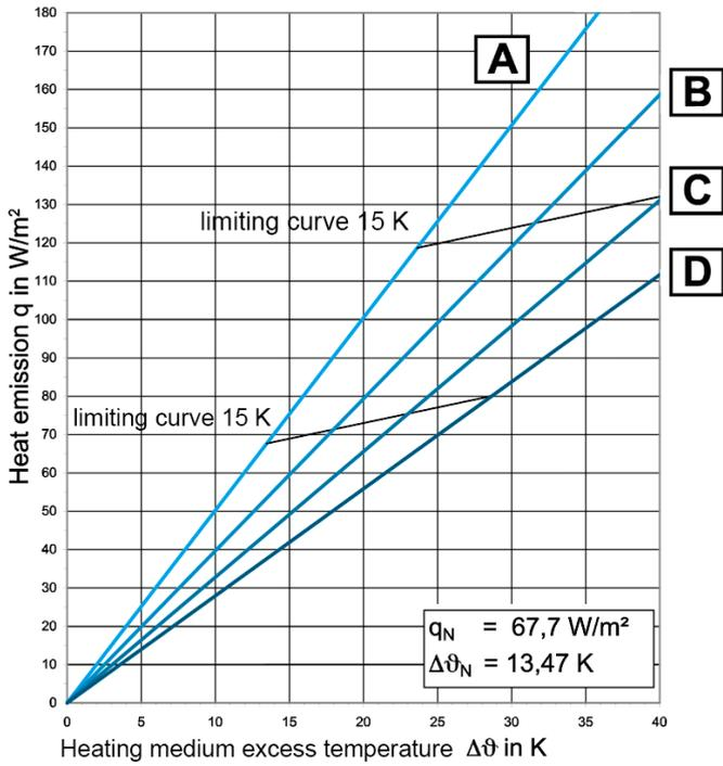
Cooling capacity of the underfloor heating
