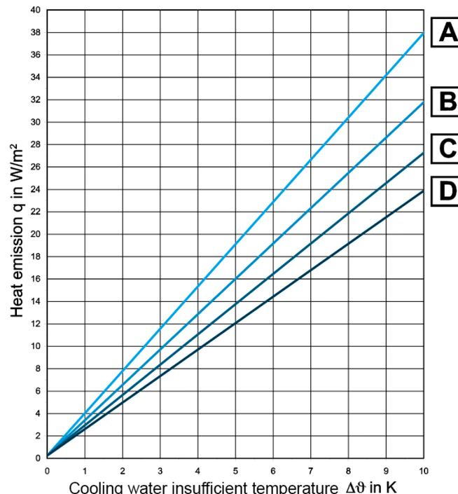
A:  $R_{\lambda,B} = 0,00$  (without floor finishing) B:  $R_{\lambda,B} = 0,05$  (with e.g. porcelain stoneware) C:  $R_{\lambda,B} = 0,10$  (with e.g. laminate flooring) D:  $R_{\lambda,B} = 0,15$  (with e.g. carpet)
