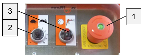
Fig. 41: Selector switch pump motor
