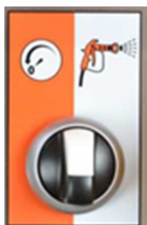
Fig. 12: Operating mode of the pump motor
