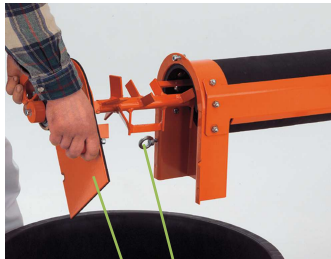
Fig. 44: Setting the mixing shaft
