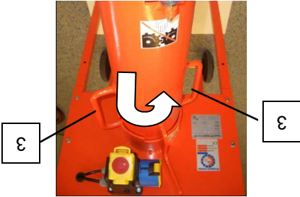
Fig. 41: Removing the mixing tube
