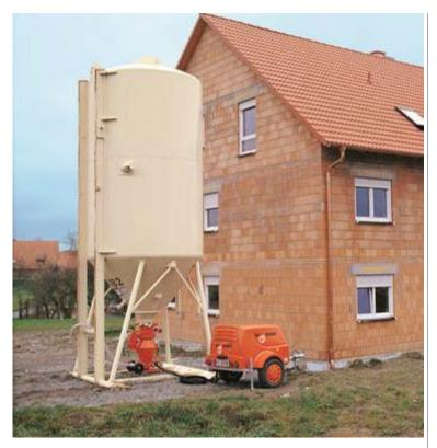
Conveyor systems can be connected to any gravity silo with a diameter of 250 mm. Gravity feeds the material into the conveying pot.
