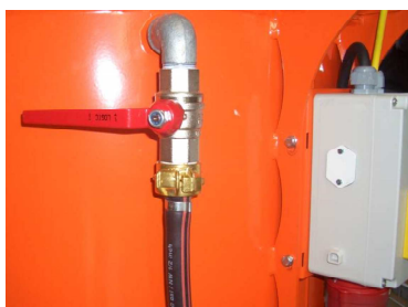
Fig. 26: Water connection
