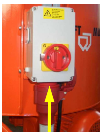
Fig. 20: Connecting the power
