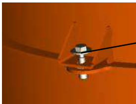
Fig. 34: Opening the protective grille
