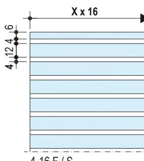
**F - cross section without acoustic processing on the rear:**
