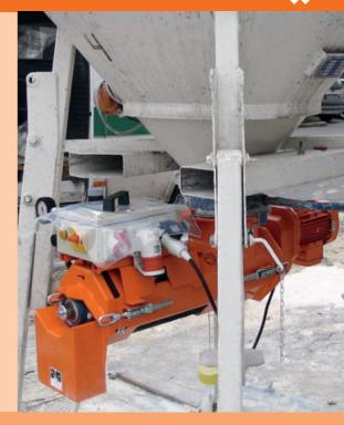
behaviour of the continuous mixer. The PFT HM 106 has a removable rubber mixing tube, which largely prevents the adherence of material. This feature makes the mixer very quick and easy to clean.
