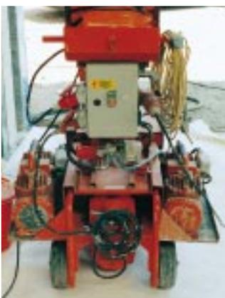
Michael Horn is not easy to satisfy with normal high-quality work. He keeps on making constant improvements that will lead to more efficiency. malerhorn processes foam mortar coats with a modified version of PFT's N2V. The modifications to the open conveying pump were Mr. Horn's own idea.
