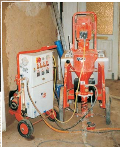
The used clay finish plaster went together well with the PFT equipment and left a neat spray pattern.
