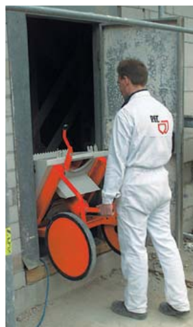
The performance of a "big one" and the manoeuvrability of a "small one" – combined in one machine. Thanks to a width of only 65 cm, the PFT G 5 fits even through narrow doors.
