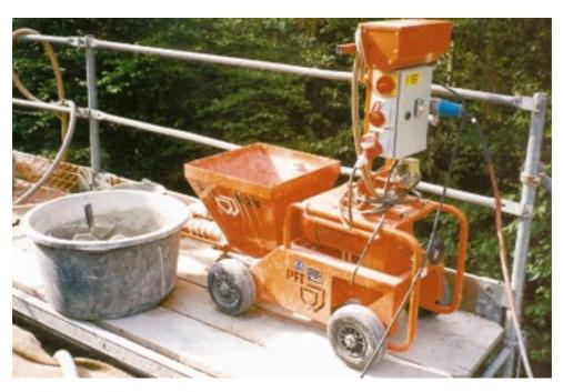
Solving problems with slowness: The open conveyor pump PFT N 2 V was set to its lowest rotation speed for the processing of the hard, grainy joint mortar.
