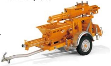
sites consists of a plaster mortar and solids-handling pump mounted onto a car chassis for the handling of grain sizes up to 8 mm. The machine components can be reset in next to no time from bag to silo feeding. The PFT adapter type HM 20 enables this combination with simultaneous use of the drivemotor and the mixing zone. The vario gear motor in the mixing
