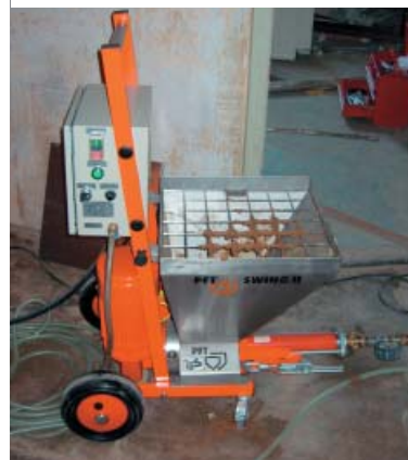
Through conveying hoses, the PFT SWING II pumps clay plaster over distances of up to 15 metres to the place of application.
