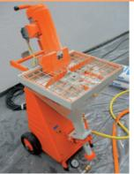
opener and the low filling height of the PFT RITMO, the bags were quickly opened and the material was neatly fed to the machine.
