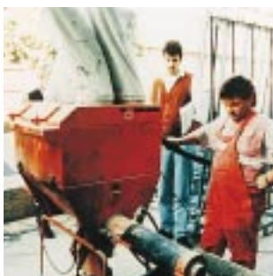
The PFT HM 2 with volume-increasing interchangeable hopper and injection hood with ventilating filter fully automatically supplied up to 30 l of mortar per minute.
