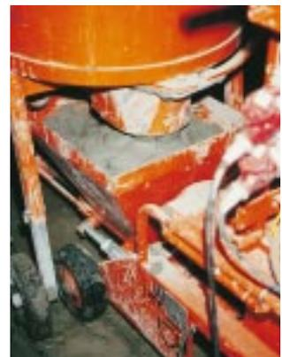
*The spraying materials were mixed with the PFT MULTIMIX and sprayed with the PFTN 2 V in one work phase.*
