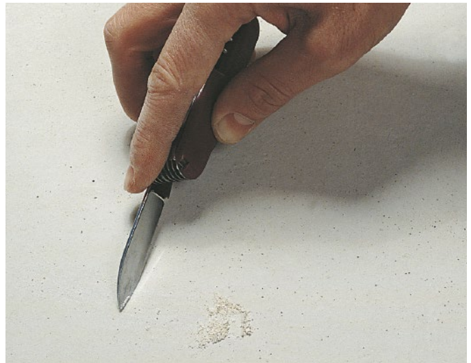
Figure 49: Inspection of the grain structure
