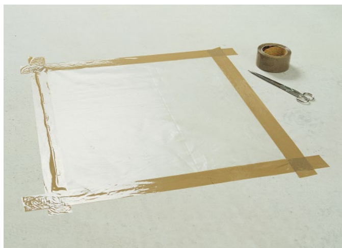
Figure 44: Initial inspection of drying with foil on the heating floor screed
