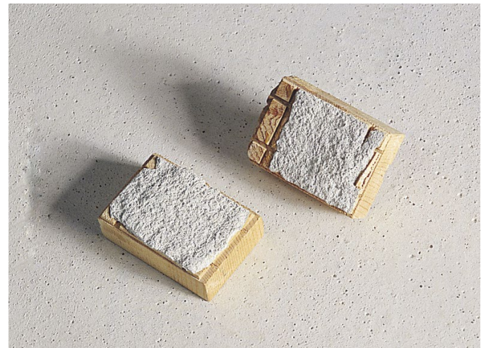
Figure 52: Parquet and screed failure patterns
