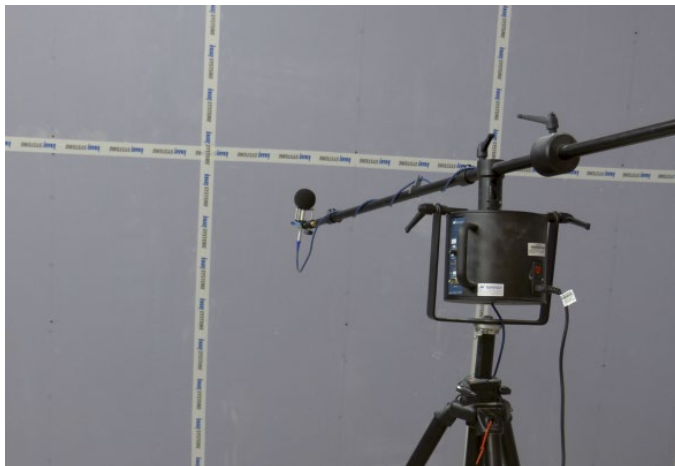
Figure 1: Airborne sound measurement
