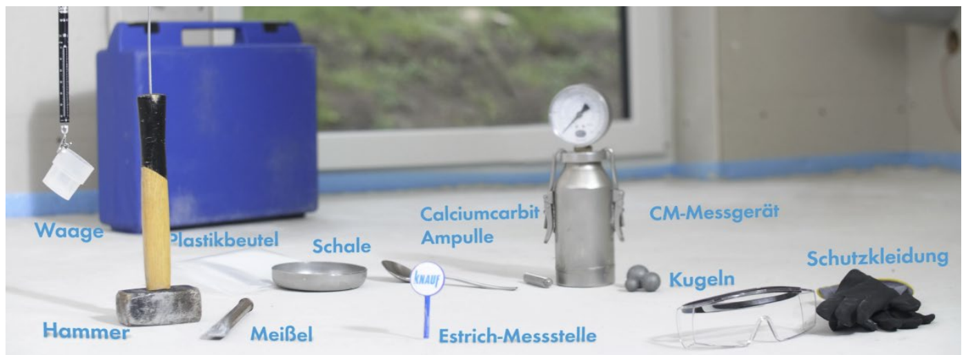
Figure 53: Testing the readiness for floor covering with the CM tester
