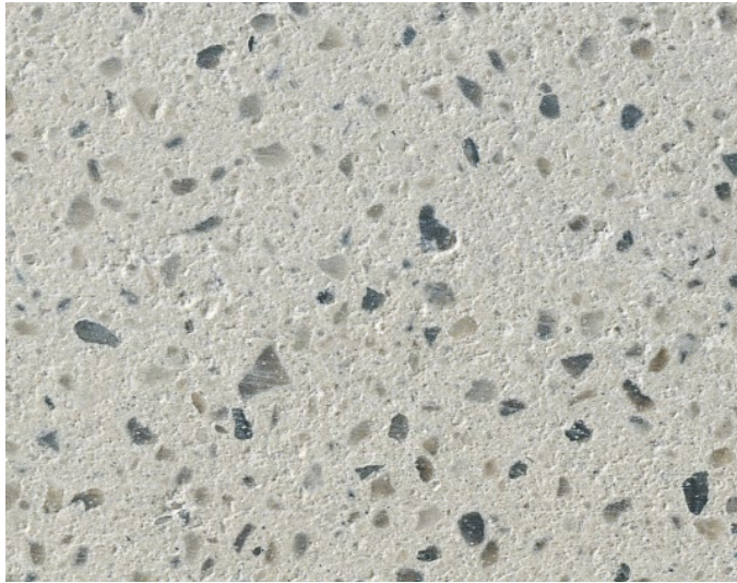
Figure 47: Flowing screed cross-section, magnified by 4
