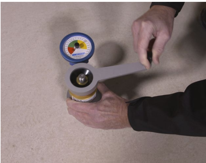
Figure 51: Test of the bond strength
